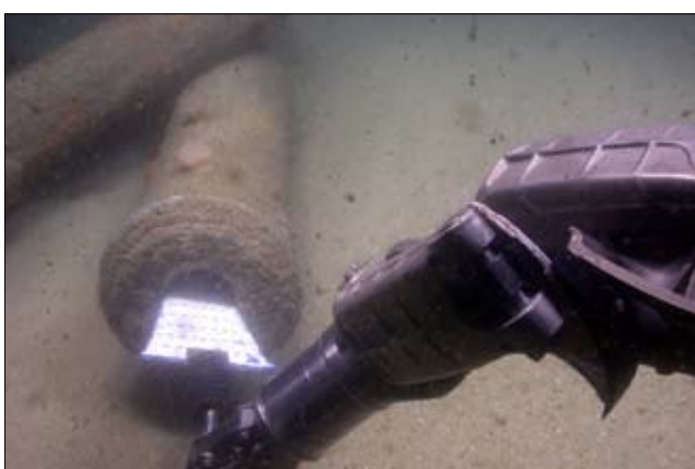
Fig. 21. ROV Zeus measuring the bore of a bronze cannon in situ.
